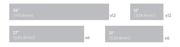
FreeLength products have a single width, 6" (152.4mm) and differing lengths. When installed with a staggered joint (see diagram below), this will give a more random pattern effect on the floor.
