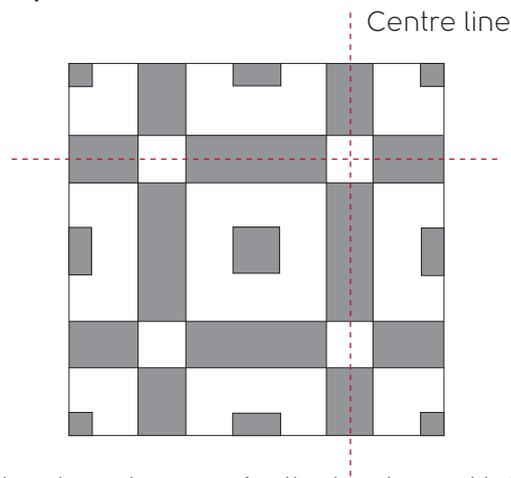
2. Install the main floor tiles, remembering to include adequate space for the border and infill if required. Then move onto installing the border, corner and infill tiles. .
