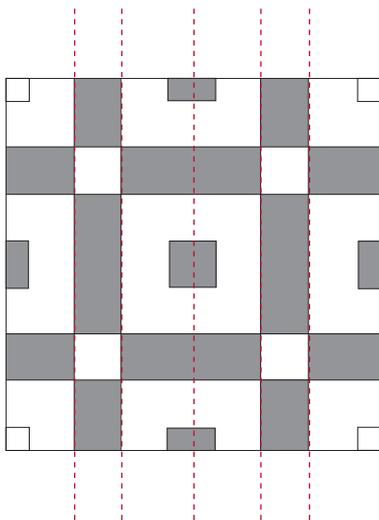
4. Install the perimeter border using the 6" infill provided making sure the border joints line up with the Brick border and floor panel joints
