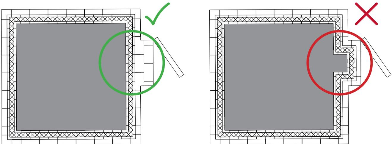
When setting out the field that is to be installed at an angle of 45°, use two straight edges or planks set at 90° to work from. This offers better initial alignment.
