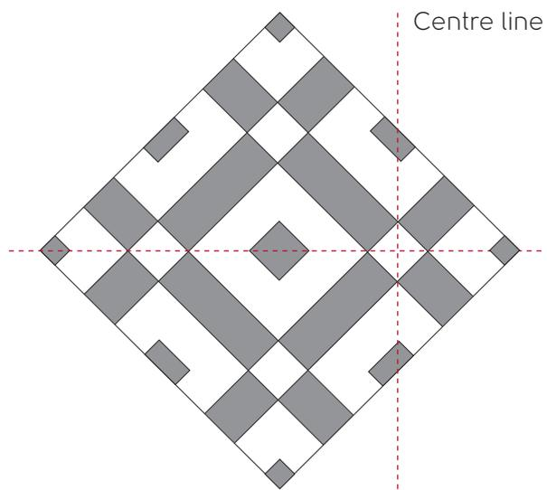
2. Install the main floor tiles, remembering to include adequate space for the border and infill if required. Then move onto installing the border, corner and infill tiles.
