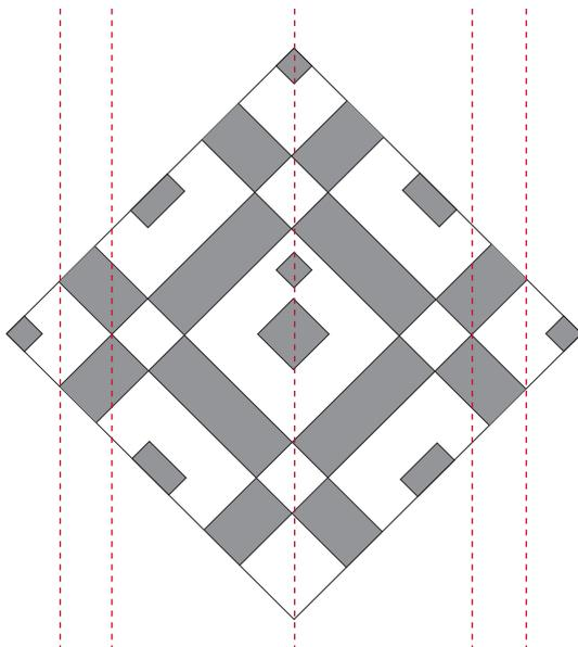
Shown below is an example floor layout. Note: The border segments for this layout do not line up with the floor panels, but it is recommended that the field tiles are only cut at the point of each diamond with the field tile. This ensures that the border always remains perpendicular to the field tiles and provides a balanced look to the overall floor.
