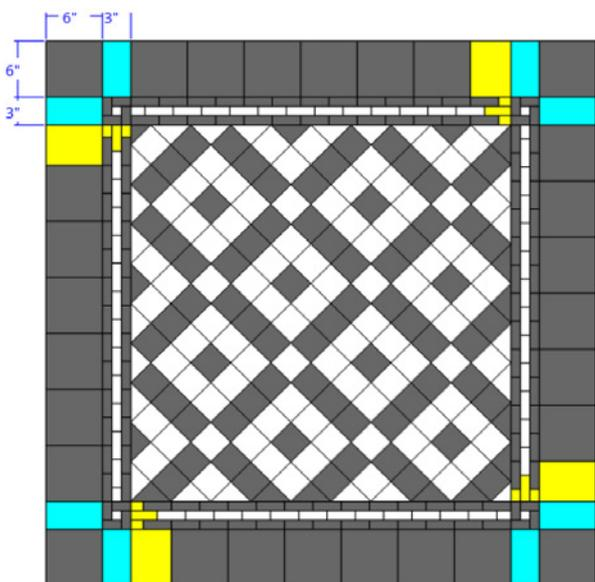
4. Install the perimeter border using the 6" infill provided making sure the border joints line up with the Brick border and floor panel joints.
